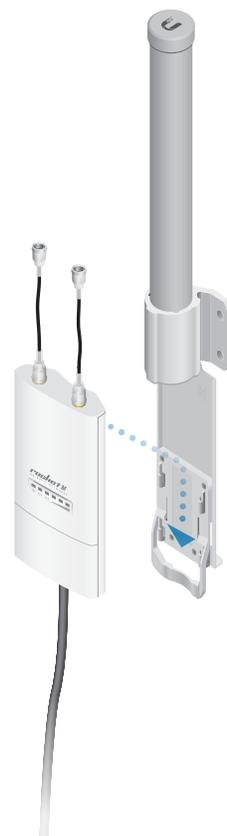
*The Rocket snaps into the built-in Rocket mount with ease.*
